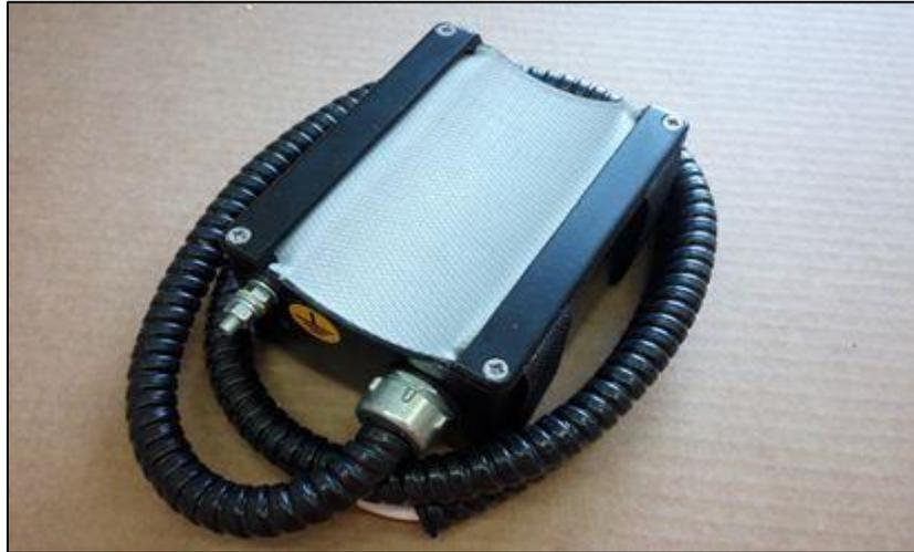
Fig. 4. Valve induction heater
