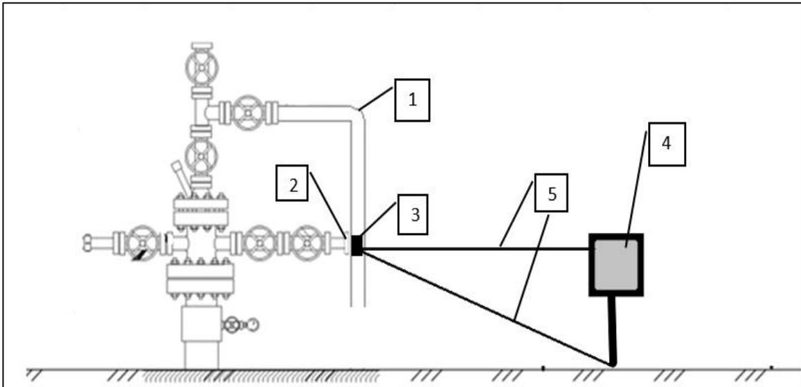
Fig. 5. Installation diagram of the valve induction heater
