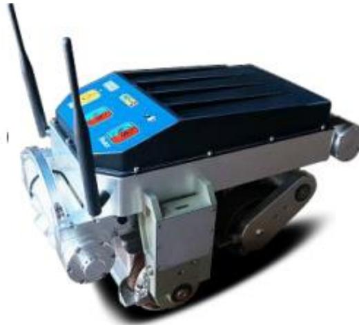
Fig. 2. Robotic complex A2072 “IntroScan”
